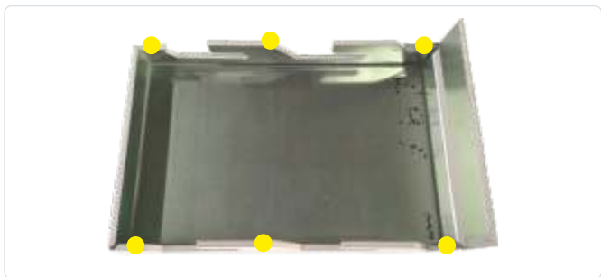
3. Folding the lateral edges and the triangular parts of the cassette to 90°
