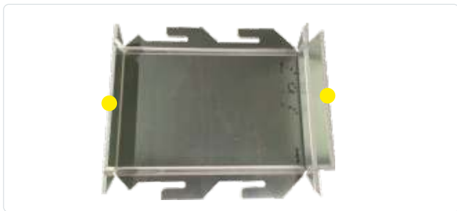
2. Folding the upper and the bottom edges of the cassettes to 90°.
